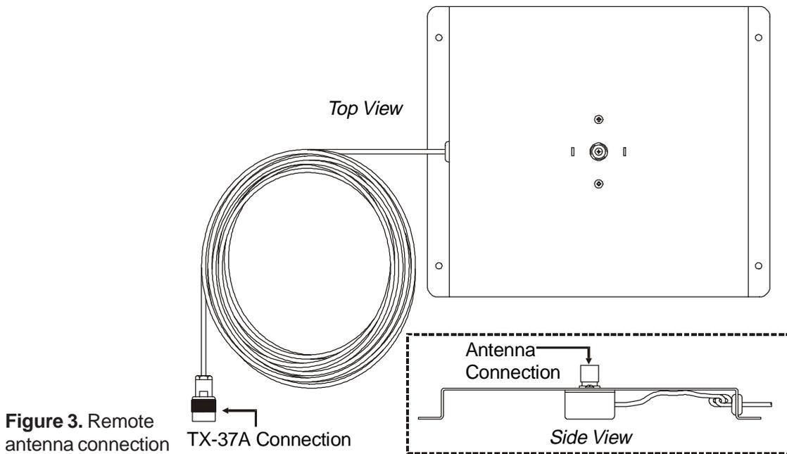
Unless the transmitter is used in a very small room, best performance is with the remote antenna placed away from the TX-37A, but as close to the receiver(s) as possible.
