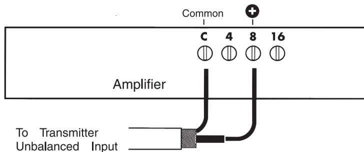
**Figure 4.** Amplifier connection
