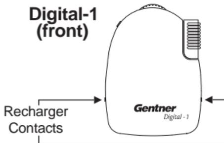
These contacts may be used in conjunction with Gentner's BC-10A for quick and easy recharging. Simply place the Digital-1 receiver in the BC-10A charger when not in use and it will automatically recharge for the next usage.
