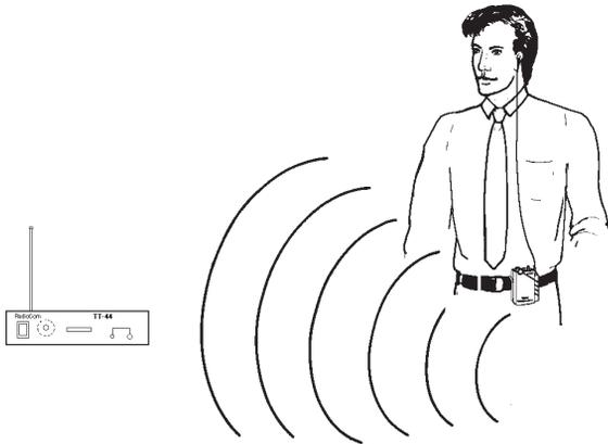
SIGNAL REACHES ANTENNA AT FULL STRENGTH WITH NO OBSTRUCTIONS.
