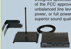
Designed specifically to help people with partial hearing loss, the TX-37A is field tunable to 37 of the FCC approved channels for ALS. Its universal input accepts mic level, balanced and unbalanced line levels, and speaker level. Signal strength is adjustable to quarter power, half power, or full power. Audio processing eliminates clipping and over-modulation while providing superior sound quality, increased intelligibility, and dynamics control. #910-402-010
